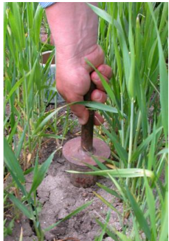
Soil moisture sampling
